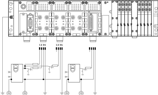
The use of decentralised devices on the fieldbus – particularly with high protection for direct machine mounting – demands a flexible power supply concept. A valve terminal with CPX-P can, in principle, supply all voltages via a single connection.
