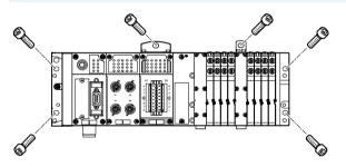
The end plates of the CPX-P terminal, the valve terminal and the pneumatic interface include mounting holes for wall mounting. Additional mountings for the CPX-P terminal are available for longer valve terminals.
